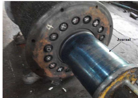
Figure 4(a) New journal fitted to the crushing roller [14]
