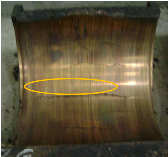
Figure 5 (c) Surface cracks
