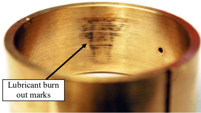
Figure 5 (a) Lubricant burnout marks
